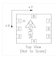
**Note:** The MEMSIC logo's arrow indicates the -X sensing direction of the device. The +Y sensing direction is rotated 90° away from the +X direction following the right-hand rule. Small circle indicates pin one (1).
