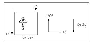
Accelerometer Position Relative to Gravity
